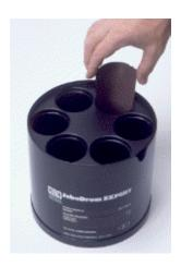
[Inserting Film Into the Expert Drum #3010]
