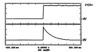
The Reset signal is on pin 10 relative to pin 22. This signal is high active. It starts the program on a defined address.
