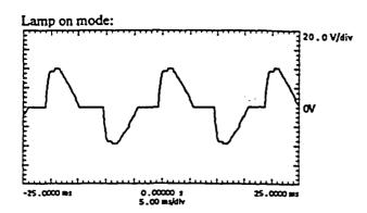
If lamp control signal goes High (12 V) so that between pin 2 and 3 is 0 V, lamp goes full power 22.5 VAC RMS. The lamp voltage can be adjusted with trimmer P1 resp. R26.
